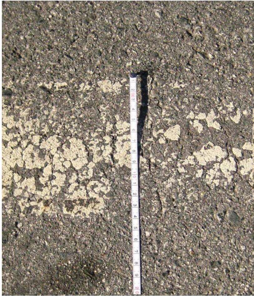
Figure 4: The measurement taken at the southernmost intersection of Family Farm Road and Portola Valley Road. Again the stripe is 14 cm (5.5 inches). Photo taken 26 Mar 2008.
